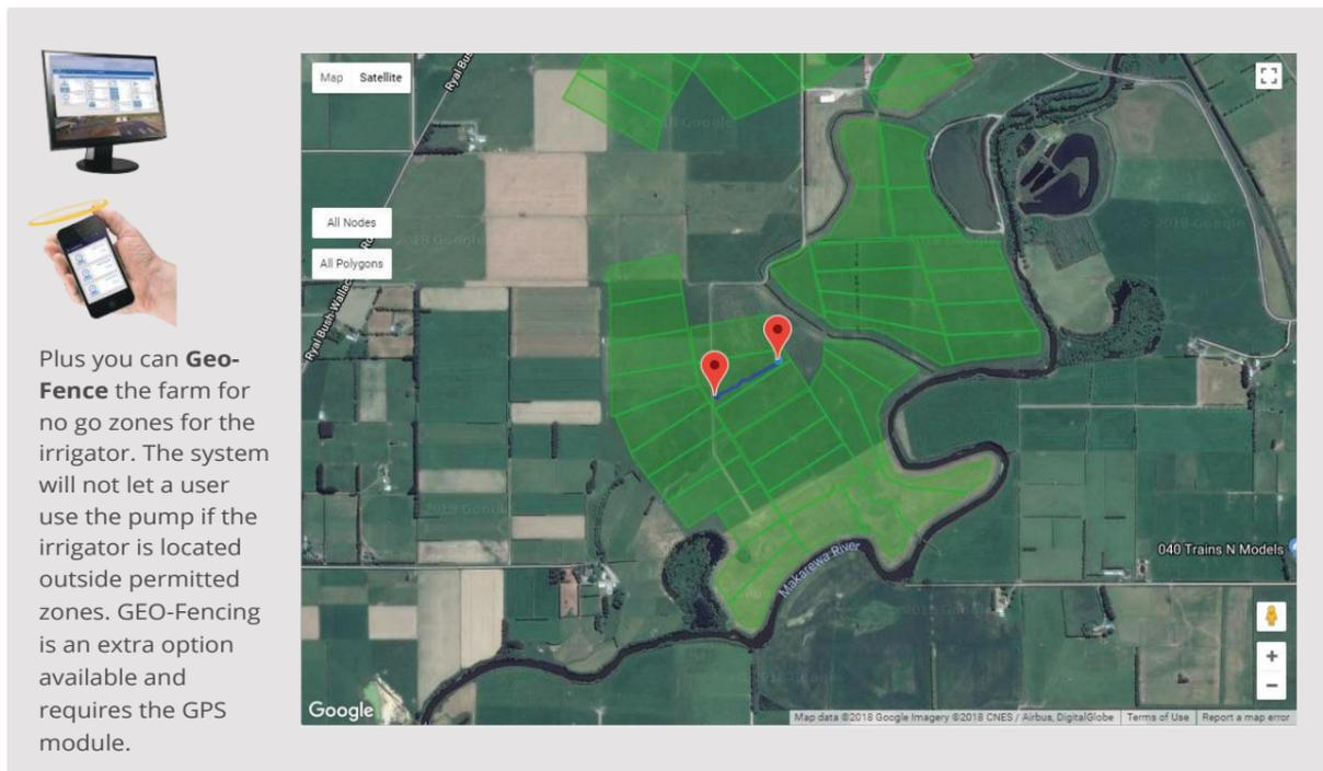
Plus you can **Geo-Fence** the farm for no go zones for the irrigator. The system will not let a user use the pump if the irrigator is located outside permitted zones. GEO-Fencing is an extra option available and requires the GPS module.
