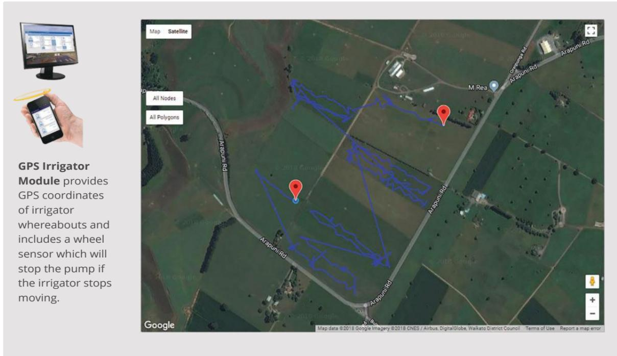
**GPS Irrigator Module** provides GPS coordinates of irrigator whereabouts and includes a wheel sensor which will stop the pump if the irrigator stops moving.
