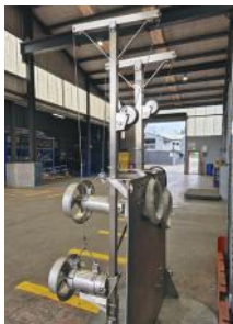
Submersible Stirrer and Lifting frame on Sump application.
