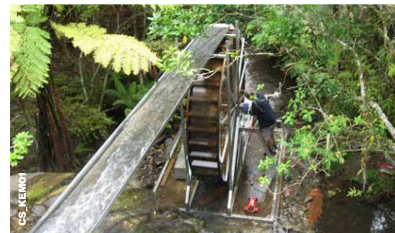
15'x2' Yardmaster Water Wheel featured construction using Kauri timber supplied by client. (see cover image)
