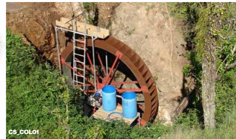
15' x 2' Yardmaster Water Wheel. Top right images shows gearbox, pulley and pump. Bottom right image shows bearings.
