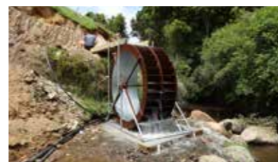
8' x 3' Yardmaster Water Wheel. Water accessed via farm creek dam and delivered via PVC to wooden flume
